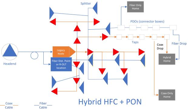
By following this combination approach, operators would incur the operating expense of running two networks, however the capital cost would be much lower than either converting to a Node + 0 HFC network or moving all of the customers to an FTTH network. This was true for low, medium, and high subscriber density plant. One large MSO CTO said, "Legacy networks stick around a long time. There is no direct reason to prompt collapsing them."
