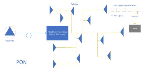
PONs have many operational advantages over HFC networks, including minimal maintenance and power requirements. One CTO reported, "All RF plant issues, such as signal leakage, no longer exist with FTTH. This enables a far more reliable network with less maintenance activities." And, "...reduced maintenance and powering saved \$2.6 million per year".
