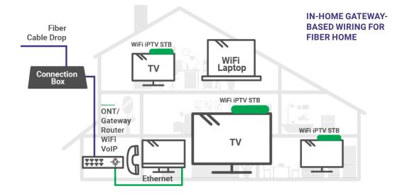
In a fiber home, the ONT terminates the outside plant optical signals, and from its associated router generates in-home signals for distribution via Wi-Fi, Ethernet, MOCA, or G.HN.
